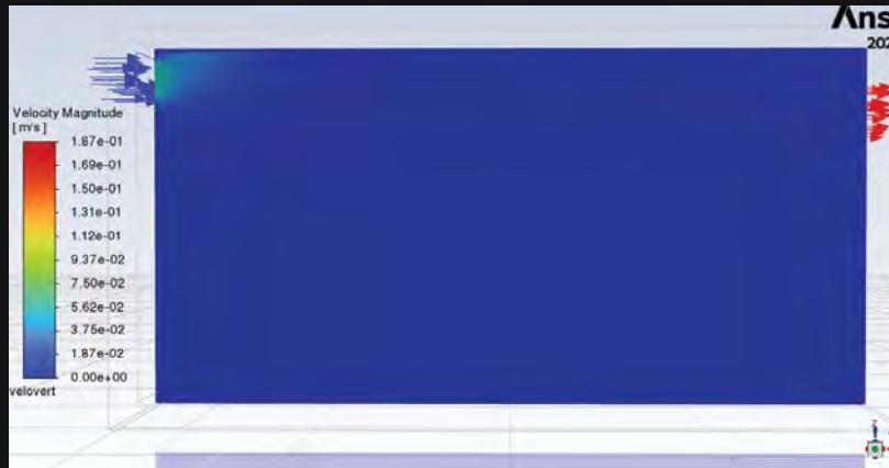
Variant 3.3 | Velocity Vertical Section
