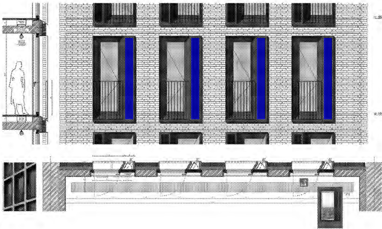
Variant 1 | Vertical, storey-high ventilation opening
